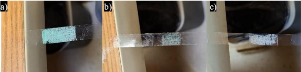
Figure 4.11 Images of the coating remains in the 3M tape after adhesion test for (a) copper azole, (b) copper quats, and (c) TiO 2 .
