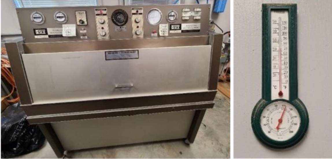
Figure 3.10 QUV accelerated weathering machine and room climate used for the test.
