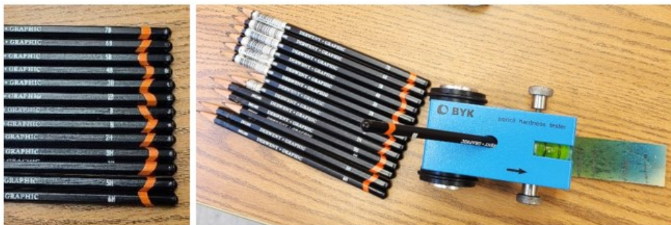
Figure 3.8 Pencil hardness kit used for ASTM 3363 standard film hardness pencil test (hardness gradually increases from 7B to 6H scale).
