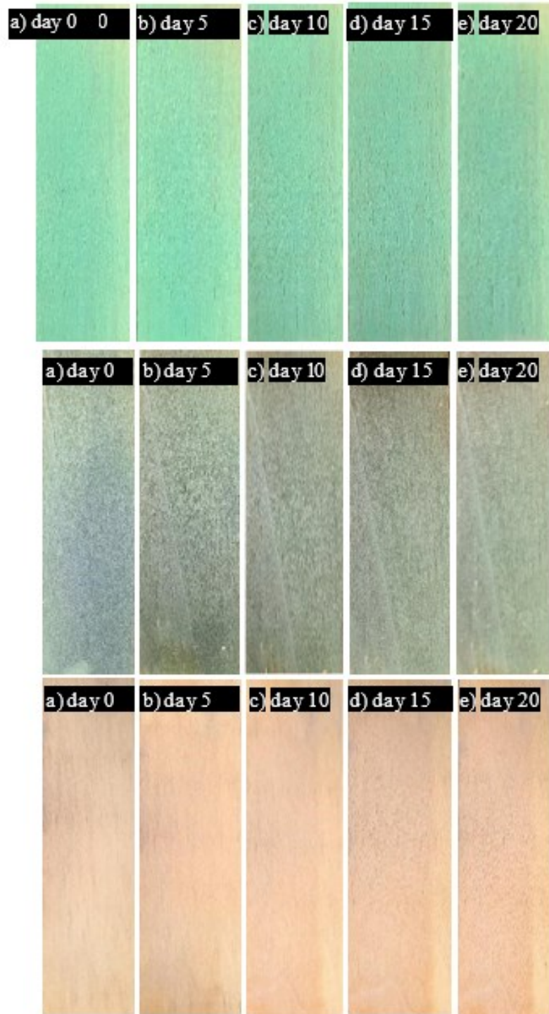
Figure 4.16 Pictures a to e: Accelerated weathering images of modified wood created by the motorized movement method (three consecutive coatings with resting) starting from day 0 to 20 with copper azole, copper quats, and titanium tetraisopropoxide as precursor solution, respectively.
