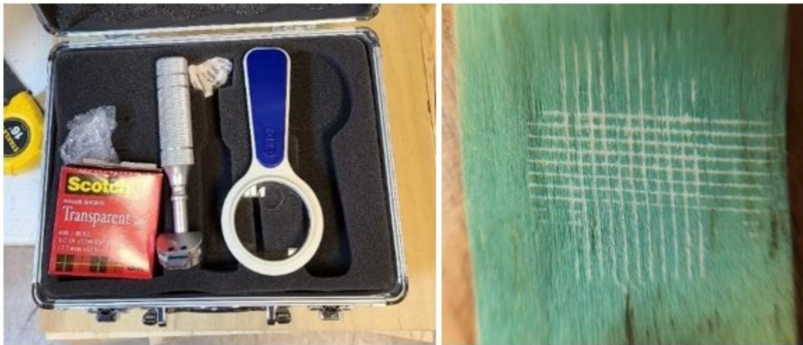
Figure 3.9 Tape test kit used and lattice pattern created on the wood substrate during ASTM D3359 measuring adhesion by tape test.
