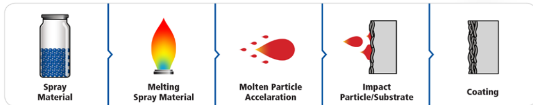
Figure 2.4 Schematic representation of thermal spray coating [28].
